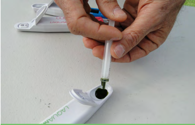
Place some drops of the extracted sap directly into the sensor.
